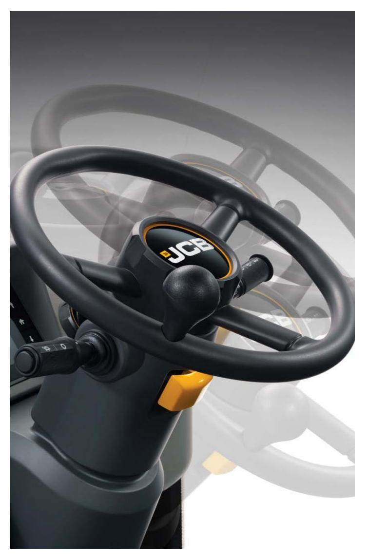
A set and forget steering column and full colour LCD display, put you comfortably in control.
